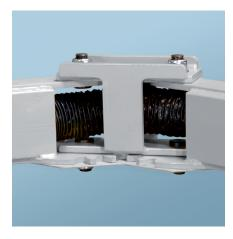
Safety guidance of the swivel arms through a smooth-running gear ring connection.
